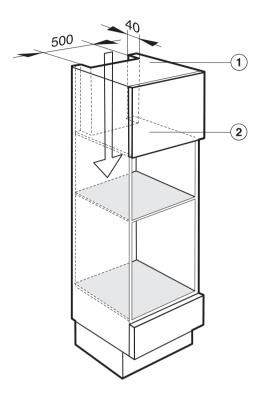
To ensure that the Combi Steam Oven has adequate ventilation, the following cut-outs measuring  $19 \ 11/16" \times 1 \ 9/16"$  (500 x 40 mm) must be made:
